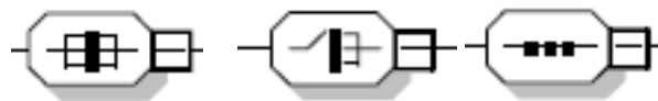
Figure B.1: The branching options in XML Schema (left to right) All , Choice and Sequence .
