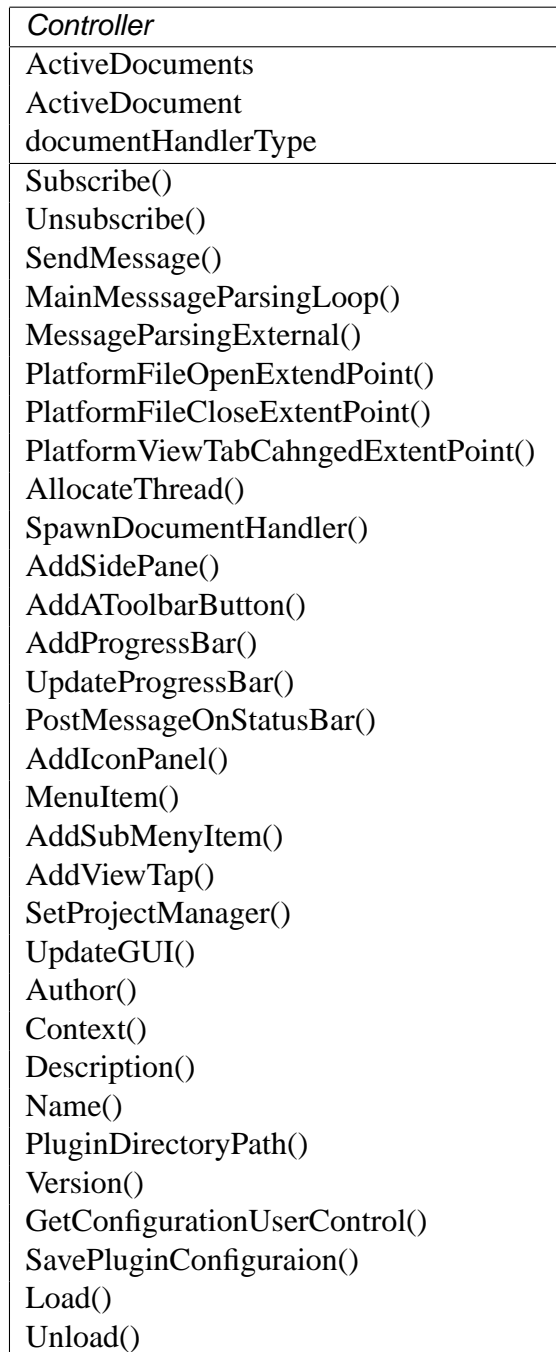
Figure 4.8: Complete class diagram of Controller
